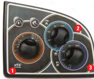
1 Selector switch (auto or manual) 2 and 3 Adjust the flow of the hydraulic line
